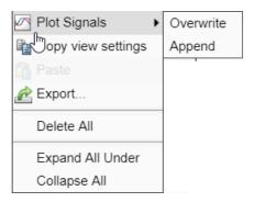
• Copy a plot view layout and the signal selection from one Sim Output to another Sim Output in the Results and Artifacts pane. Select the Sim Output to copy from. Then, click Transfer Signal View
